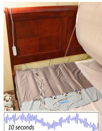
Fig. 7. The hydraulic bed sensor with 10 seconds of data. The high amplitude, low frequency signal is breathing. The high frequency component is the ballistocardiogram of the heart.
